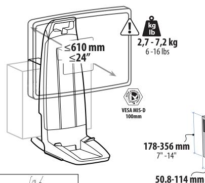
**CAUTION:** This stand is intended for use only within the weight ranges indicated. Use with products heavier than the maximum weights indicated may result in instability causing personal injury or equipment damage.
